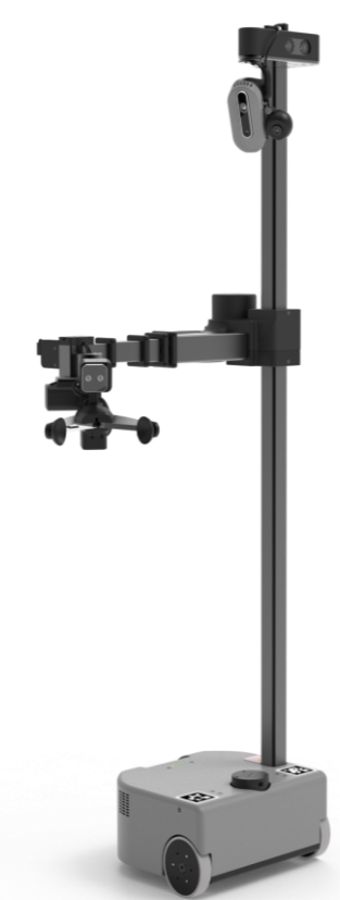
Target control platform: Hello Robot Stretch 3 [7]
